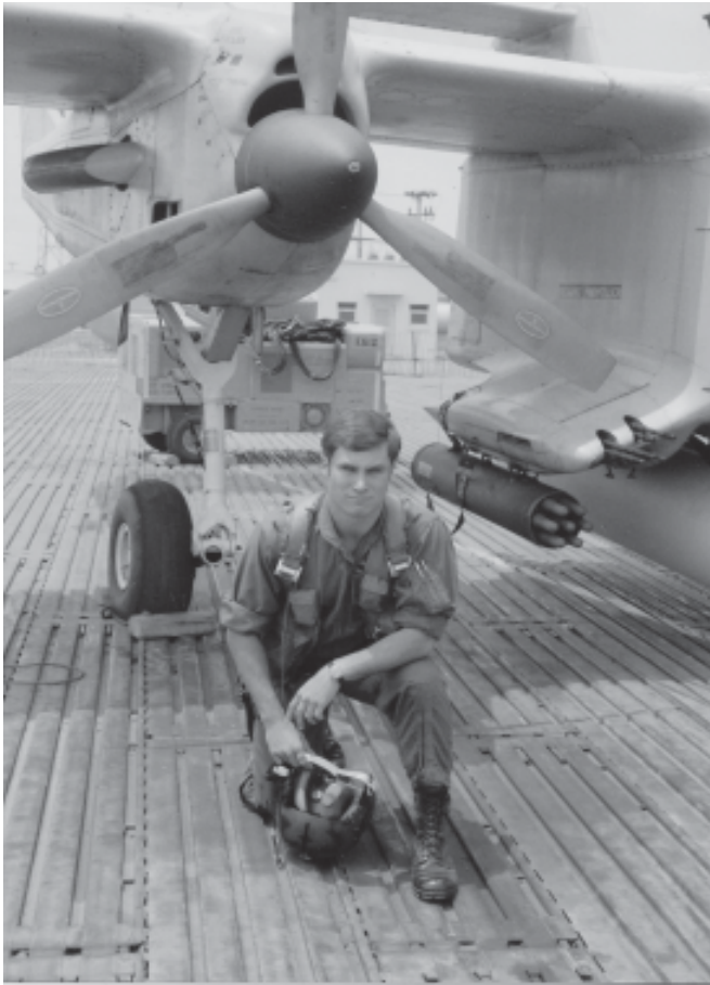
Jim Kidd, showing engine, main landing gear, and weapons stations on the OV-10 close air support aircraft. Note the PSP parking ramp surface. PSP is pierced steel planking, which was developed during World War 2.
