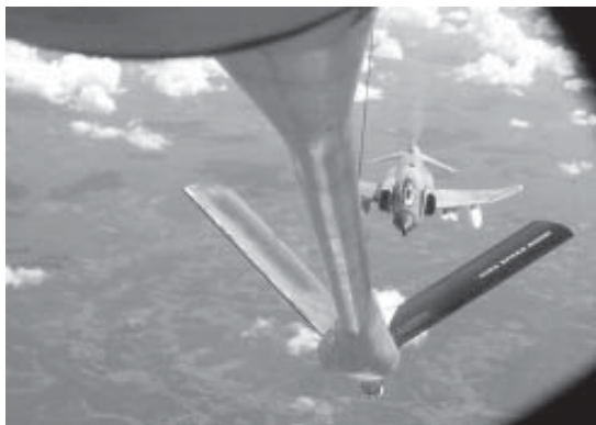
Below: F-4 fighter approaches refueling boom on a KC-135, somewhere over Eastern Thailand, 1971. (photo, Bill Tilton)
