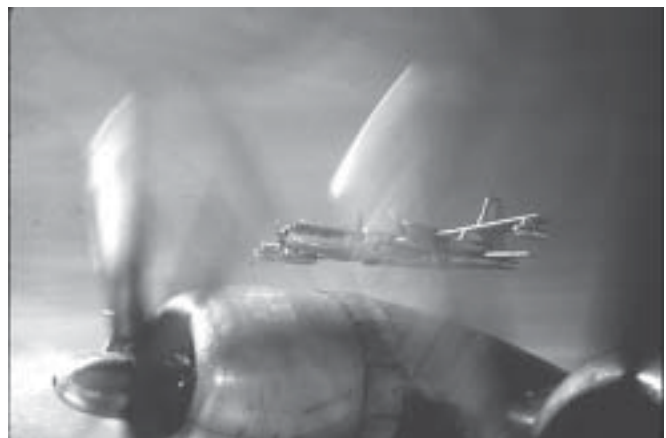
KB-50J wingman as seen from the co-pilot's window. Note auxiliary J-47 engines and wingtip refueling reel pods; also a pod in the tail. The propeller disc was 18 feet in diameter (do you have an 18 foot room in your house?)
